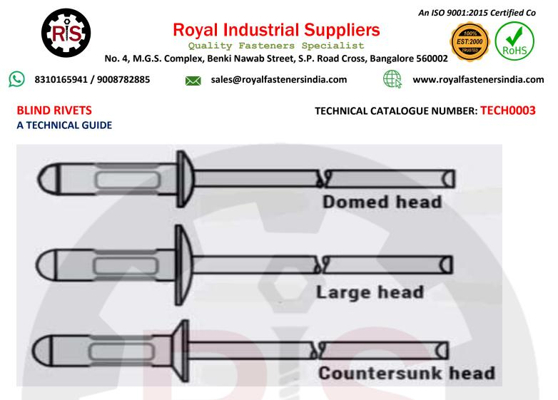
The most popular is the Dome Head, whose lower profile head is approximately twice the diameter of the rivet body. This provides adequate bearing surface for nearly all applications.
